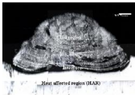
Fig. 1: Macrostructure of clad layer of laser clad Inconel 617 with Ni-10%Al premixed clad powder at cladding speed of 5.3 mm/s.
